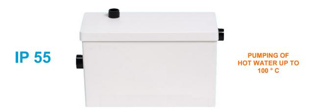
Unlike normal macerator units which have a limit to the water temperature they can handle, with **Geyser** the hot temperature of the water doesn't cause any overheating of the motor as it sits outside the tank.
