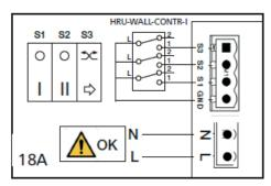
Connection of 2 HRU-WALL units with a single HRU-WALL-CONTR-I controller
