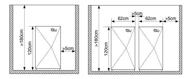
Design dimensions of the heat pump from the top
