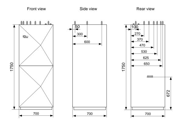
Design dimensions of the heat pump with integrated boiler from the front
