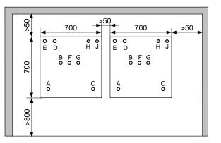
H, J – openings for electrical connection cables.
