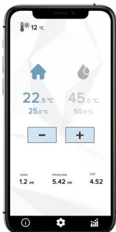
IGLU® Aleut geothermal heat pumps are controlled via the IGLU® Home app. It allows to control the device and monitor the operating parameters of the heating system, electricity consumption, thermal energy produced and instantaneous or seasonal coefficient of performance in real time.
