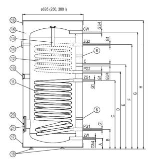
SB; SBZ; SW; SWZ Cylinder construction (4001; 5001)
