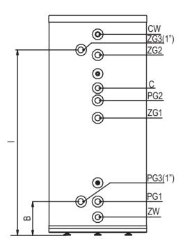
Before starting the heat exchanger, an optical inspection of the device connection and the correct assembly according to the diagrams must be carried out. All connections, including those that were factory-assembled (connection nozzles of the electric heater, magnesium anode, inspection opening cover), must be checked for tightness upon startup and resealed in case of leaks. The heat exchanger must be filled with water:
