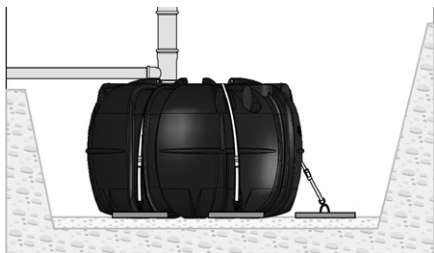
Anchoring with anchor plates.
